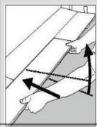
5. Lift planks (together with the previous laid in the same row) lightly up (about 30 mm), push it against the row in front and then put it down. Adjust the distance to the wall to 10 mm when three rows are completed. Proceed installation as described above until reaching the opposite wall.
