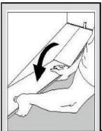
4. Place short end of the plank at an angle against the previous installed plank and fold down. Ensure that the plank is positioned on the integral locking strip of the plank in the previous row.
